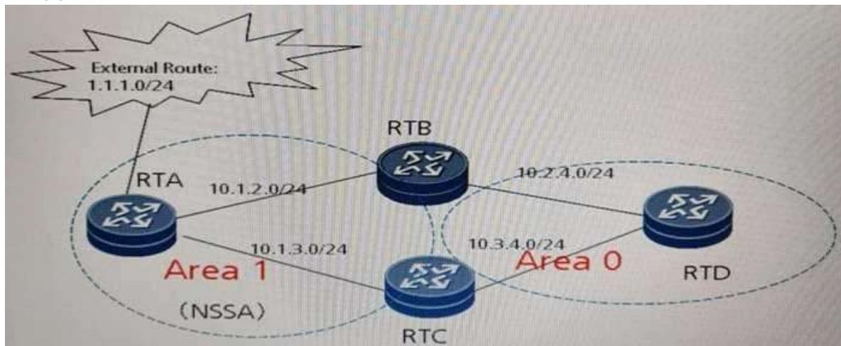
As shown in the figure, external route 1.1.1.0/24 is imported to RTA that is located in the NSSA area. RTD is a backbone area router. RTB and RTC are both area border router (ABRs). OSPF configuration are as follows.
